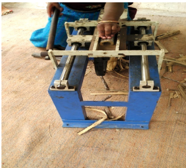
Figure 2. Bamboo cuttings made into chips using hand-operated machine
