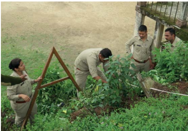
Contouring using a Frame Method
